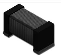
This new design is coil with a very stable and high quality ferrite core and tiny size  $(5.1 \times 10^{-5})$ 2.3 x 2.4mm) and high sensitivity in low frequency range (20-40kHz). Those pieces are winding with thin copper wire up to 12 µm and its inductances range is 40-270 mH. Besides, it has good frequency and temperature behaviour and can be served with "custom" electrics characteristics according requirements of hearing aid devices manufacturers.
