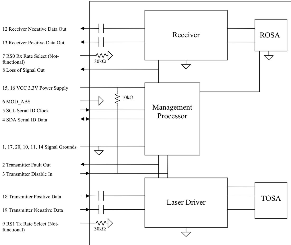
Figure 1 SFP+ optical transceiver functional block diagram
