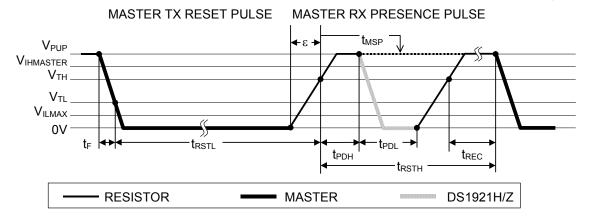
After the bus master has released the line it goes into receive mode (RX). Now, the 1-Wire bus is pulled to  $V_{PUP}$  via the pull-up resistor or, in case of a DS2480B driver, by active circuitry. When the threshold  $V_{TH}$  is crossed, the DS1921H/Z waits for  $t_{PDH}$  and then transmits a presence pulse by pulling the line low for  $t_{PDL}$ . To detect a presence pulse, the master must test the logical state of the 1-Wire line at  $t_{MSP}$ .
