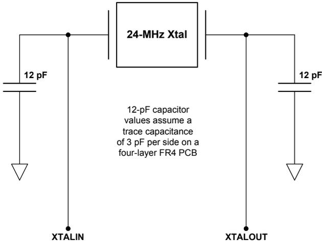
The NX2LP requires a 24 MHz ( $\pm 100$  ppm) signal to derive internal timing. Typically, a 24 MHz (20 pF, 500  $\mu$ W, parallel-resonant fundamental mode) crystal is used, but a 24 MHz square wave from another source can also be used. If a crystal is used, connect its pins to XTALIN and XTALOUT, and also through 12 pF capacitors to GND. If an alternate clock source is used, apply it to XTALIN and leave XTALOUT open.
