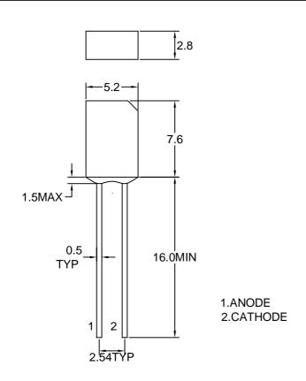
NOTE:1.All dimension are In millimeters tolerance Is ±0.25 unless otherwise noted 2. Specifications are subject to change without notice
