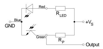
Note: Customer has to select suitable resistors for chosen supply voltage. Pull-up resistor  $R_{\rm p}$  could be e.g. 10  $k\Omega$  depending on desired output. Forward voltage of LED is 1.3 V and LED current should be 10 mA (depending on application liquid).  $R_{\rm LED}$  can be calculated as follows (e.g. for  $V_{\rm S}$ =12 V):
