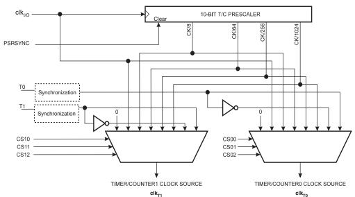
Figure 16-2. Prescaler for Timer/Counter0 and Timer/Counter1<sup>(1)</sup>
