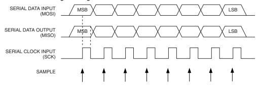
For characteristics of the SPI module see "SPI Timing Characteristics" on page 309.
