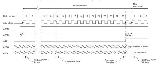
Figure 23-5. ADC Timing Diagram, Single Conversion
