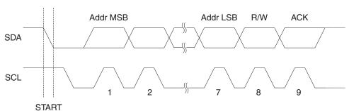
Figure 21-4. Address Packet Format
