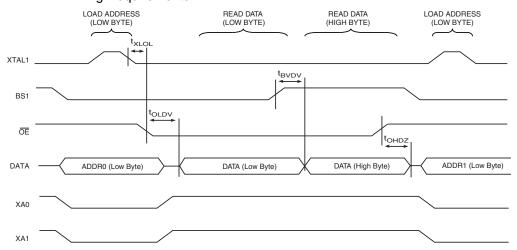
Note: 1. The timing requirements shown in Figure 28-6 (i.e., t<sub>DVXH</sub>, t<sub>XHXL</sub>, and t<sub>XLDX</sub>) also apply to reading operation.
