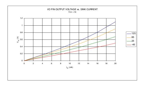
**Figure 29-8.** I/O Pin Output Voltage vs. Sink Current ( $V_{CC} = 5 \text{ V}$ ).
