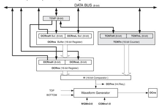
Figure 15-4. Output Compare Unit, Block Diagram
