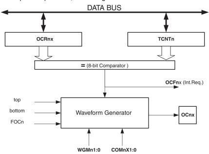
Figure 17-3. Output Compare Unit, Block Diagram
