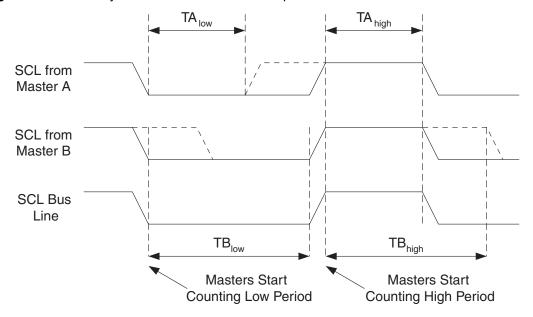
Figure 21-7. SCL Synchronization Between Multiple Masters
