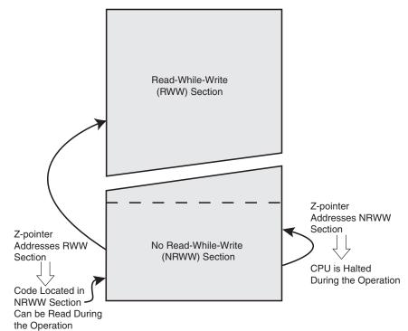
Figure 26-1. Read-While-Write vs. No Read-While-Write
