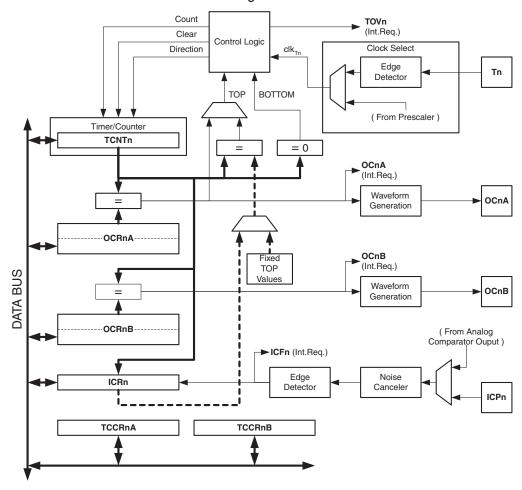
Figure 15-1. 16-bit Timer/Counter Block Diagram<sup>(1)</sup>
