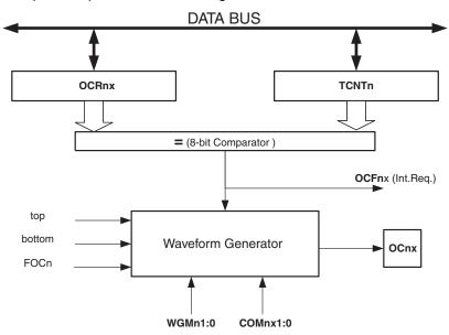
Figure 14-3. Output Compare Unit, Block Diagram
