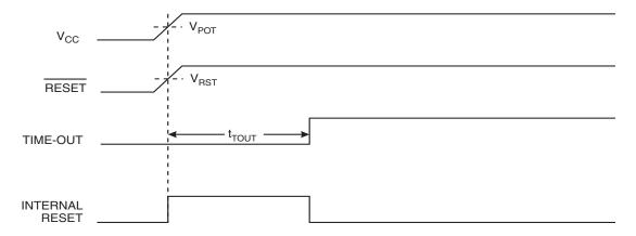
Figure 10-3. . MCU Start-up, RESET Extended Externally
