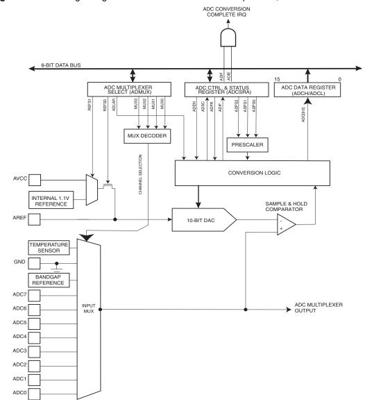
Figure 23-1. Analog to Digital Converter Block Schematic Operation,
