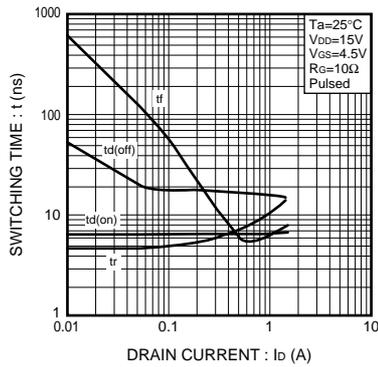
Fig.1 Switching Characteristics
