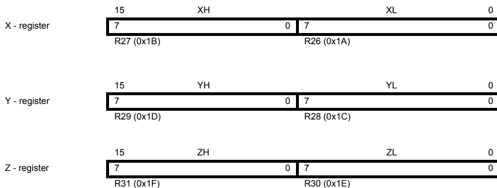
Figure 6-3. The X-, Y-, and Z-Registers
