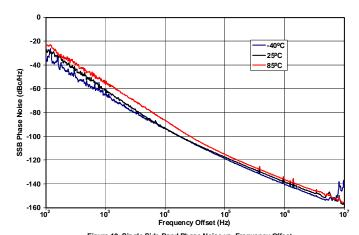
Figure 10. Single Side Band Phase Noise vs. Frequency Offset (Vctrl = 5V)
