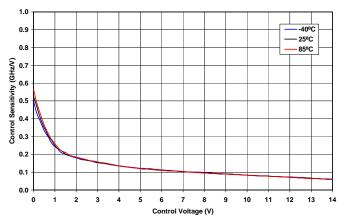
Figure 7: Frequency Sensitivity vs. Control Voltage and Temperature - RF Port
