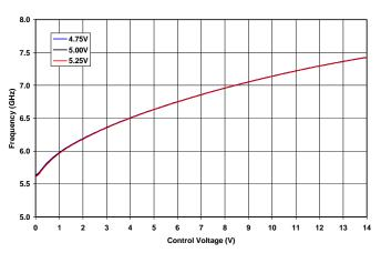
Figure 3: Frequency vs. Control Voltage and Supply Voltage - RF Port
