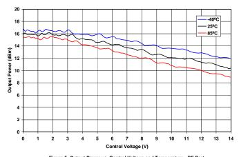
Figure 5: Output Power vs. Control Voltage and Temperature - RF Port
