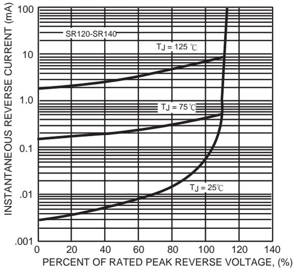
FIG. 3B - TYPICAL REVERSE CHARACTERISTICS
