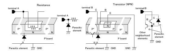
Example of simple structure of IC
