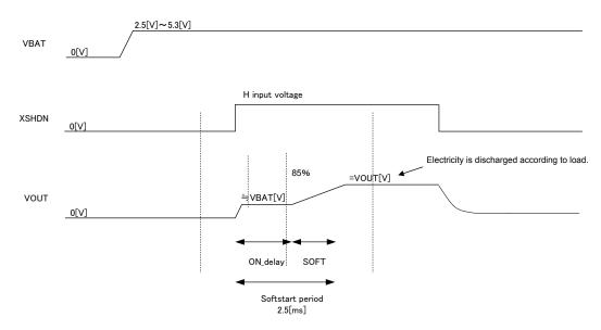
Fig.14 DC/DC converter start wave form
