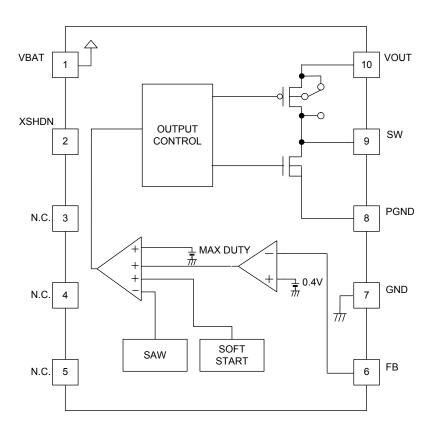
Fig.13 Block Diagram
