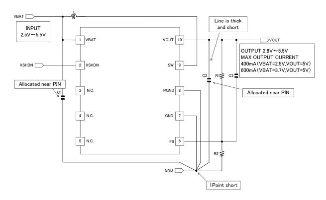
Fig.19 Application circuit figure
