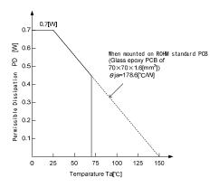
Fig.20 Permissible Dissipation
