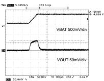
Fig.11 Load transient response wave form
