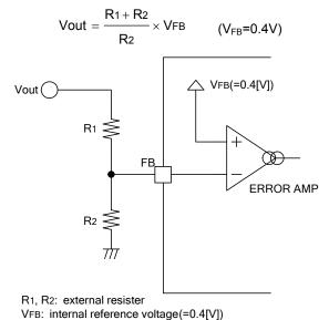
Fig.15 Output voltage setting
