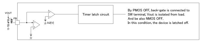
Fig.18 Ground short circuit protection function
