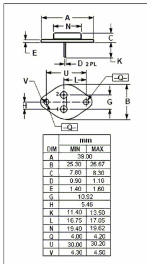
**isc Silicon NPN Power Transistor****BDY90A****ELECTRICAL CHARACTERISTICS**T<sub>c</sub>=25°C unless otherwise specified
