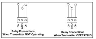
Relay output '1' provides a longer momentary output (approx ½ second) this may be removed by adding Link 6 on the PCB. The outputs are driven from a Microcontroller and can be customised to specific requirements.
