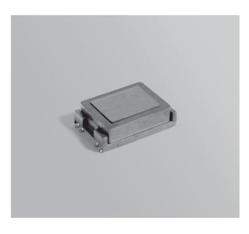
The FA2786-BL was developed specifically for the Texas Instruments TPS68000 Phase Shift Full Bridge CCFL Controller. It is designed for use in cold cathode fluorescent lamp power supplies operating at frequencies up to 100 kHz.
