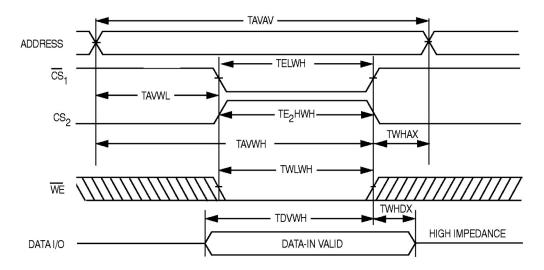
Note: The internal write time of the memory is defined by the overlap of  $\overline{CS1}$  Low and  $\overline{CS2}$  HIGH and  $\overline{W}$  LOW. Both signals must be actived to initiate a write and either signal can terminate a write by going in actived. The data input setup and hold timing should be referenced to the actived edge of the signal that terminates the write. Data out is high impedance if  $\overline{OE} = V_{H}$ .
