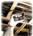
☐ Measurement reading reverses automatically when the display is flipped open to ensure readability.
