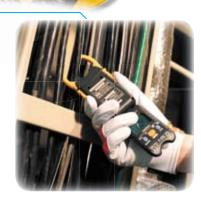
Sometimes it's easier to clamp the target wire at an angle.
