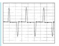
Inverters, office equipment, AC adapters - most load current waveforms are distorted. Current meters that display average rectified RMS values does not allow you to obtain accurate RMS measurements.
