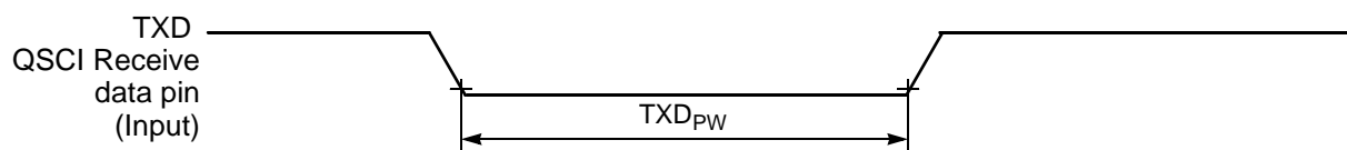
Figure 10-13 TXD Pulse Width
