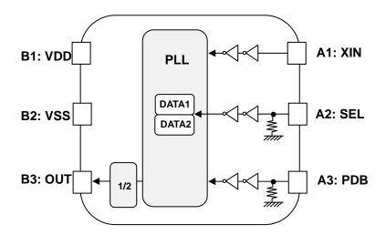
VDD=3.3V, Ta=25°C, XIN=27.0000MHz 38.0000MHz output (OUT=XIN $\times$ (76/27)/2) as SEL=L 36.0000MHz output (OUT=XIN $\times$ (8/3)/2) as SEL=H
