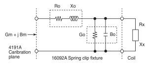
Gm + jBm: Measured admittance [S] Ro + jXo: Residual impedance [Ω] Go + jBo: Stray admittance [S] Rx + jXx: Unknown impedance [Q]
