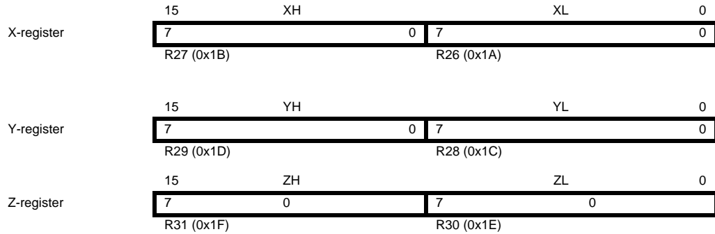
Figure 6-3. The X-, Y-, and Z-registers
