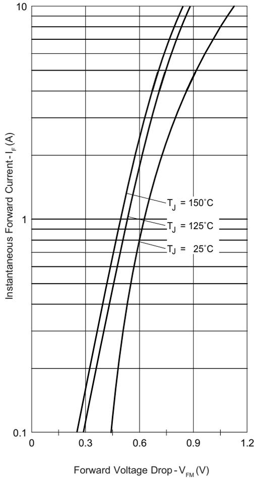
Fig. 1 - Maximum Forward Voltage Drop Characteristics
