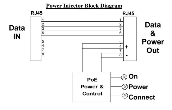
**Description of LED Functions for Power Injector**
