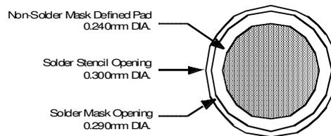
Figure 8. Recommended Non-Solder Mask Defined Pad Illustration
