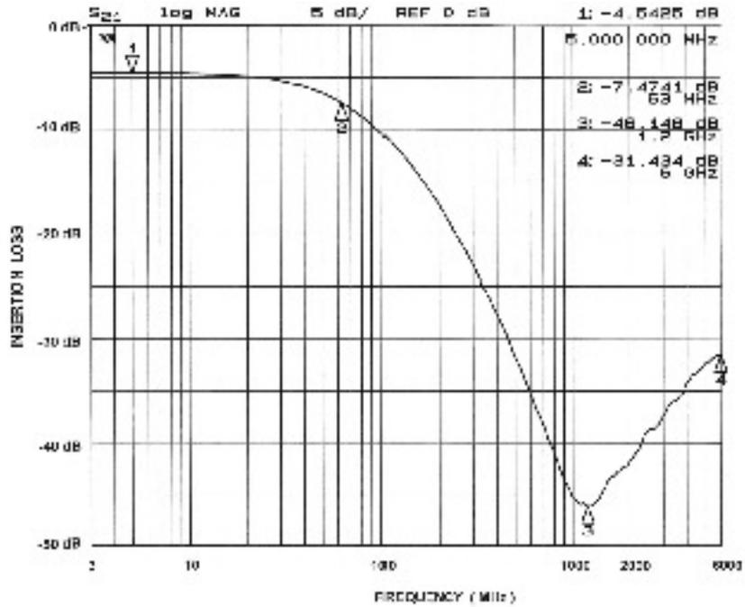
Figure 3. Microphone Circuit (A5-C5) EMI Filter Performance
