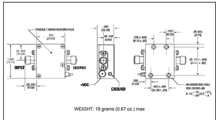
\* Dimensions are inches (millimeters)  $\pm 0.015$  (0.38) unless otherwise specified.
