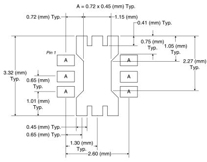
Figure 2. PCB Solder Mask (Top View)
