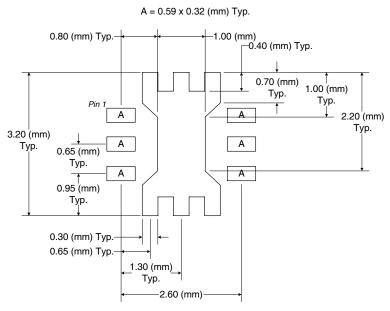
Figure 1. PCB Metal Land Pattern (Top View)
