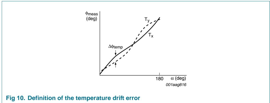
**Fig 10. Definition of the temperature drift error**
