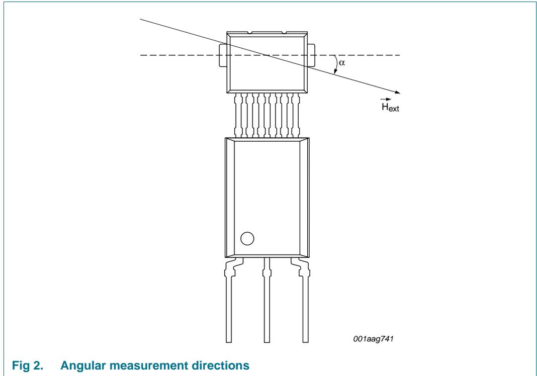
**Fig 2. Angular measurement directions**
