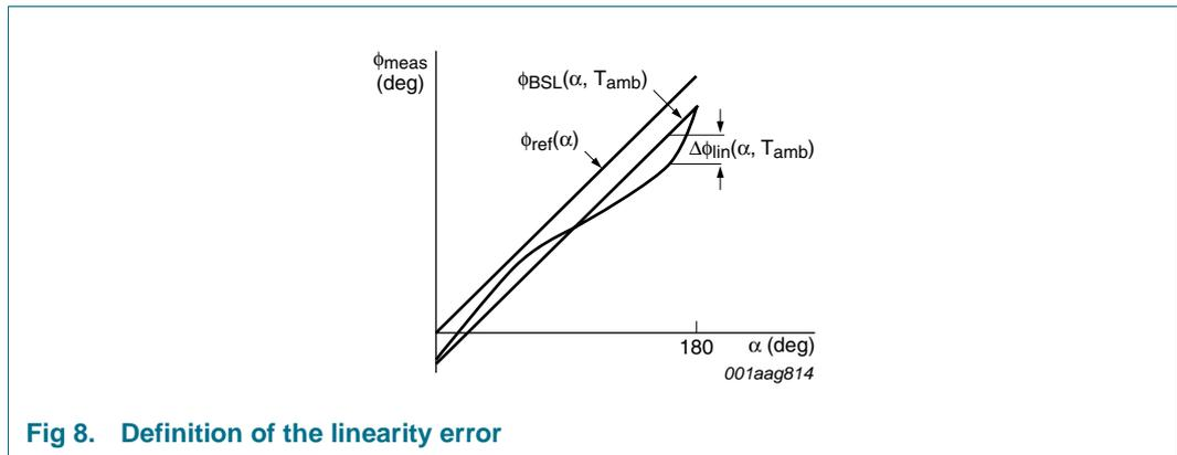
Fig 8. Definition of the linearity error
