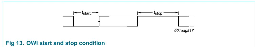
Fig 13. OWI start and stop condition
