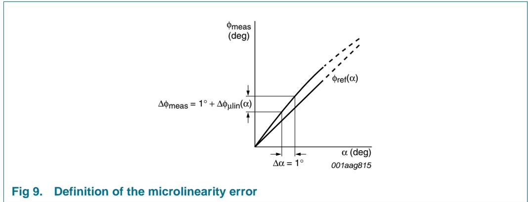
**Fig 9. Definition of the microlinearity error**
