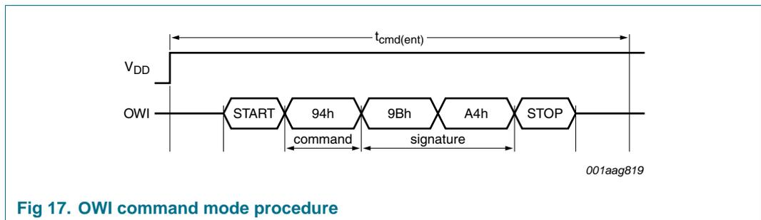
Fig 17. OWI command mode procedure
