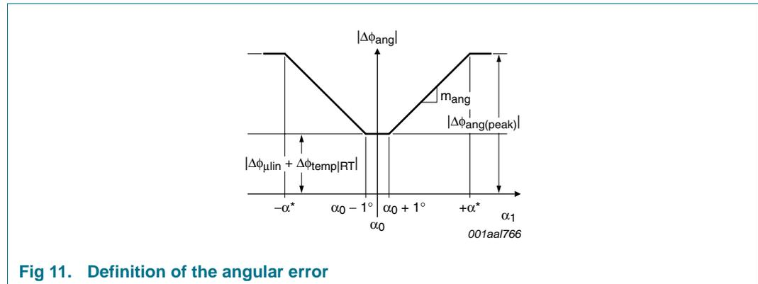
**Fig 11. Definition of the angular error**
