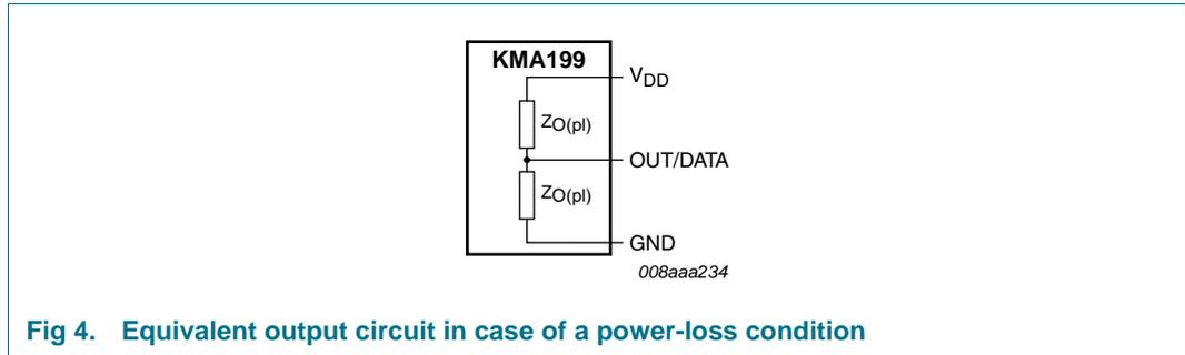
Fig 4. Equivalent output circuit in case of a power-loss condition
