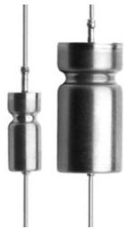
Vishay ST represents a major breakthrough in wet tantalum capacitor technology. Its unique cathode system provides the highest capacitance per unit volume. The design facilitates a doubling of capacitance, lower ESR and higher ripple current rating compared with conventional wet tantalum products. Moreover, the ST has the capacitance stability of a solid tantalum capacitor and there are no circuit impedance restrictions.
