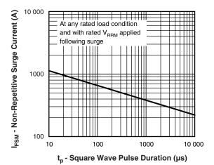
Fig. 7 - Maximum Non-Repetitive Surge Current (Per Leg)
