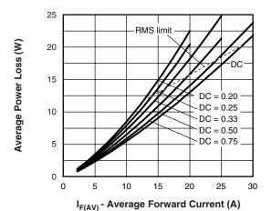
Fig. 6 - Forward Power Loss Characteristics
