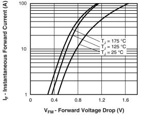
Fig. 1 - Maximum Forward Voltage Drop Characteristics
