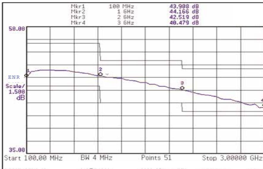
The NFP1003 Noise Source features high ENR output in a small SMT package, ideal for military and other harsh environment applications.
