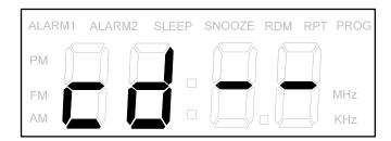
2) When CD closed, it begins to read TOC. It will enter STOP state after read over, if there is no operation in 5s, and then return to time display.
