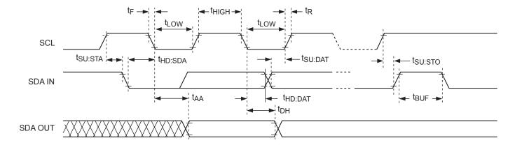
Figure 1. I<sup>2</sup>C Bus Timing Characteristics
