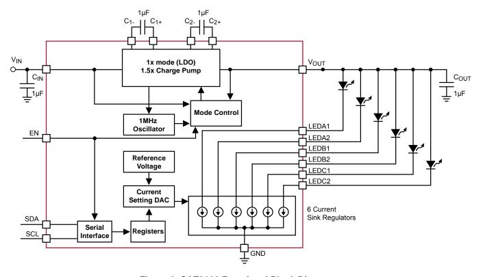
Figure 2. CAT3626 Functional Block Diagram
