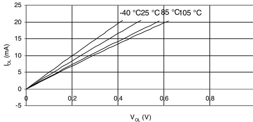
**Figure 27-18. I/O Pin Sink Current vs. Output Voltage ( $V_{CC} = 2.7V$ )**
