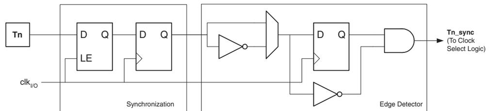
The synchronization and edge detector logic introduces a delay of 2.5 to 3.5 system clock cycles from an edge has been applied to the Tn/T0 pin to the counter is updated.
