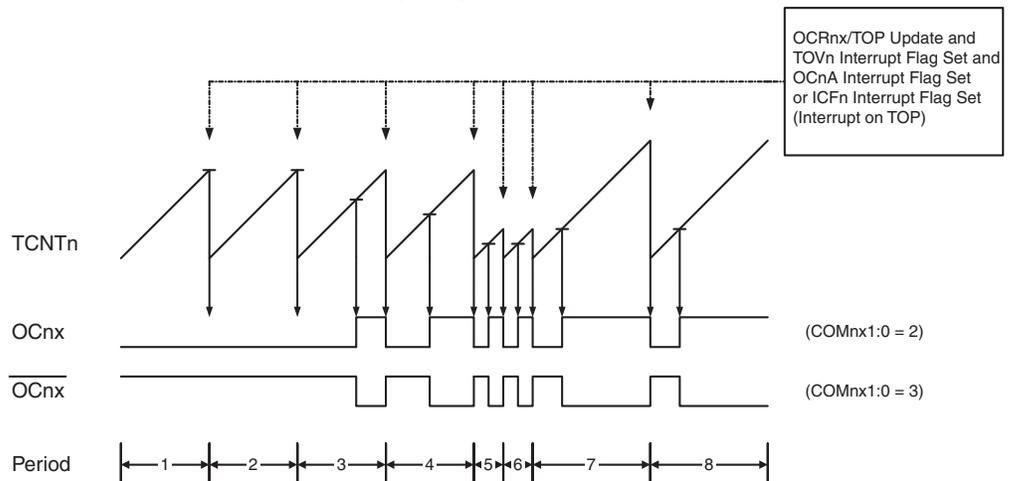
The Timer/Counter Overflow Flag (TOVn) is set each time the counter reaches TOP. In addition the OCnA or ICFn Flag is set at the same timer clock cycle as TOVn is set when either OCRnA or ICRn is used for defining the TOP value. If one of the interrupts are enabled, the interrupt handler routine can be used for updating the TOP and compare values.
