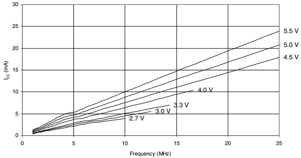
**Figure 27-3.** Active Supply Current vs.  $V_{CC}$  (Internal RC Oscillator, 8 MHz)
