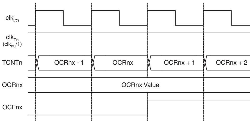
[Figure 15-11](#) shows the same timing data, but with the prescaler enabled.
