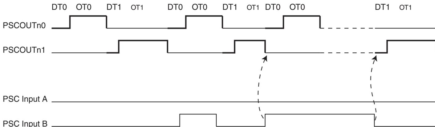
PSC Input B is take into account during DT1 and OT1 only. It has no effect during DT0 and OT0. When PSC Input B event occurs, PSC releases PSCOUTn1, jumps and executes DT0 plus OT0 and then waits for PSC Input B inactive state. Even if PSC Input B is released during DT0 or OT0, DT0 plus OT0 sub-cycle is always completely executed.
