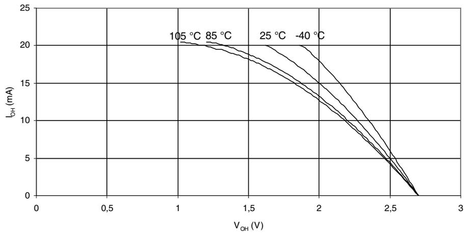
**Figure 27-17.** I/O Pin Sink Current vs. Output Voltage ( $V_{CC} = 5V$ )
