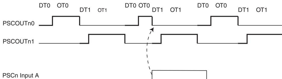
The output frequency is modulated by the occurrence of significant edge of retriggering input.
