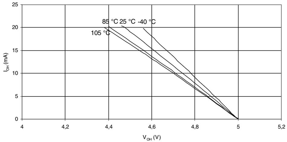
**Figure 27-16.** I/O Pin Source Current vs. Output Voltage ( $V_{CC} = 2.7V$ )
