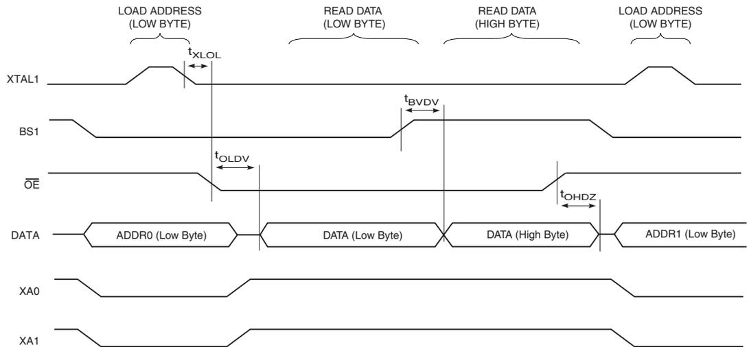
Note: 1. The timing requirements shown in Figure 26-5 (i.e.,  $t_{DVXH}$ ,  $t_{XHXL}$ , and  $t_{XLDX}$ ) also apply to reading operation.
