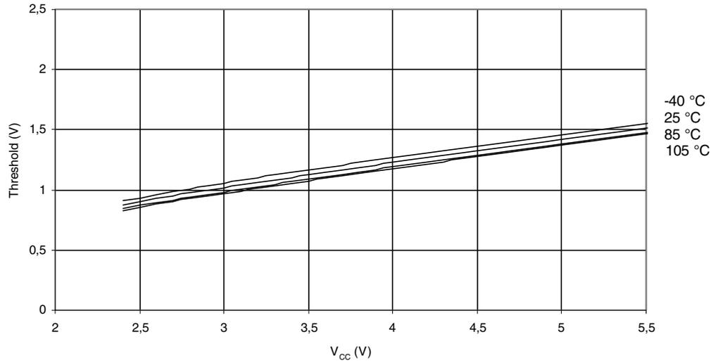
**Figure 27-21.** I/O Pin Input Hysteresis Voltage vs.  $V_{CC}$
