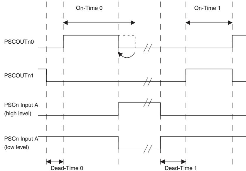
Note: This example is given in “Input Mode 1” in “2 or 4 ramp mode” See Figure 16-20. for details.
