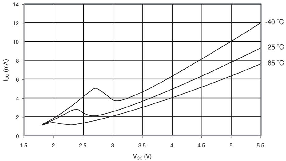
27.11 Current Consumption in Reset and Reset Pulse width
