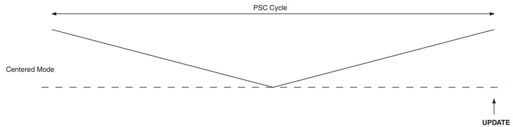
Ramps illustrate the output of the PSC counter included in the waveform generators. Centered Mode is like a one ramp mode which count down up and down.
