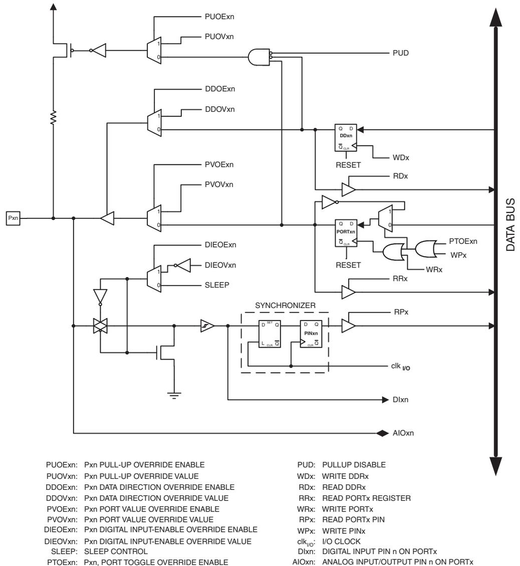
Note: 1. WR<sub>x</sub>, WP<sub>x</sub>, WD<sub>x</sub>, RR<sub>x</sub>, RP<sub>x</sub>, and RD<sub>x</sub> are common to all pins within the same port. clk<sub>I/O</sub>, SLEEP, and PUD are common to all ports. All other signals are unique for each pin.
