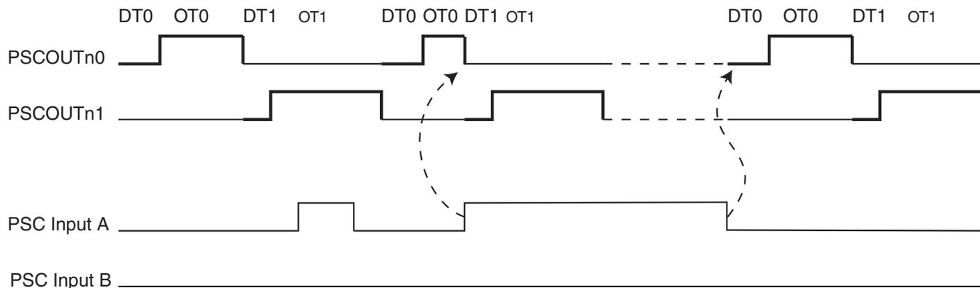
PSC Input A is take into account during DT0 and OT0 only. It has no effect during DT1 and OT1. When PSCn Input A event occurs, PSC releases PSCOUTn0, jumps and executes DT1 plus OT1 and then waits for PSC Input A inactive state. Even if PSC Input A is released during DT1 or OT1, DT1 plus OT1 sub-cycle is always completely executed.
