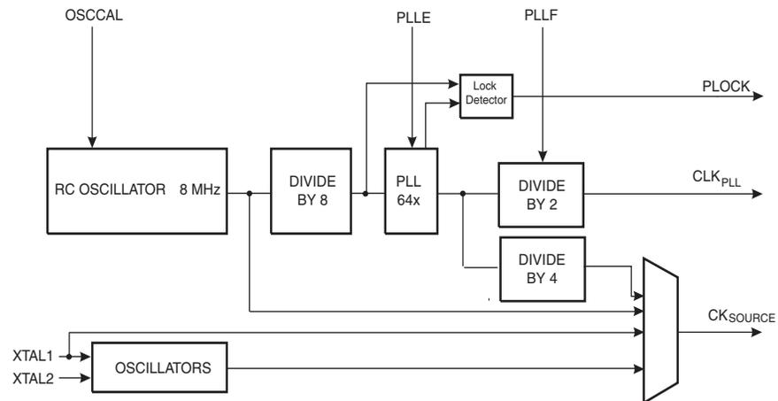
**Figure 7-5. PCK Clocking System AT90PWM2B/3B**
