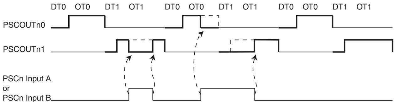
**Figure 16-27.** PSC behaviour versus PSCn Input A or Input B in Fault Mode 4
