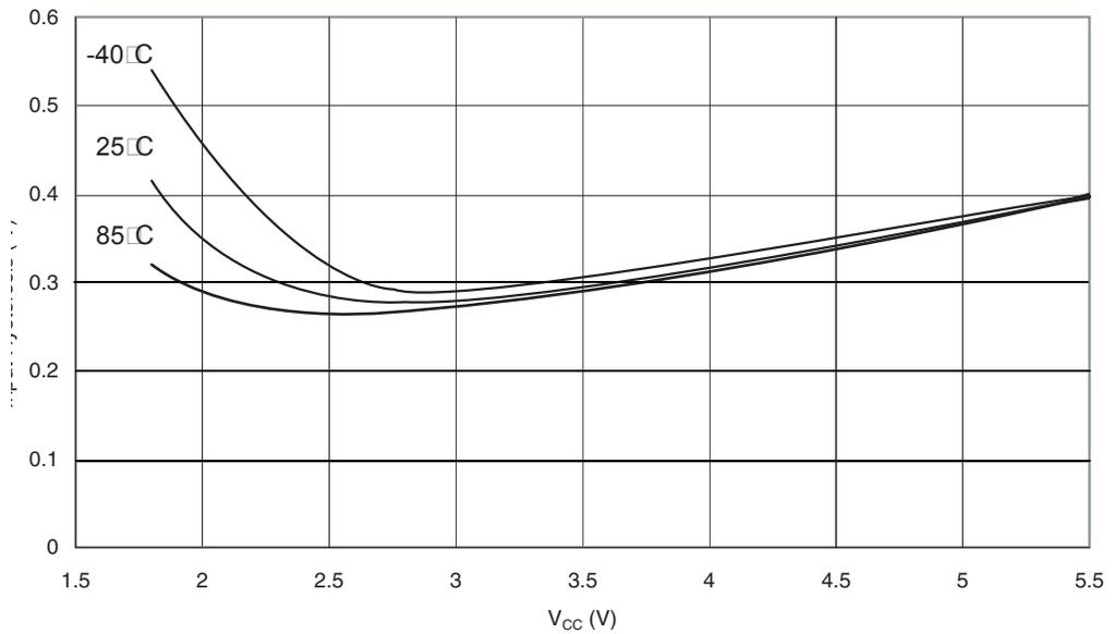
**Figure 27-22.** Reset Input Threshold Voltage vs.  $V_{CC}$  ( $V_{IH}$ , Reset Pin Read As '1')
