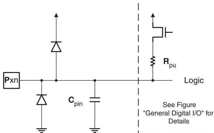
All registers and bit references in this section are written in general form. A lower case “x” represents the numbering letter for the port, and a lower case “n” represents the bit number. However, when using the register or bit defines in a program, the precise form must be used. For example, PORTB3 for bit no. 3 in Port B, here documented generally as PORTx<sub>n</sub>. The physical I/O Registers and bit locations are listed in “[Register Description for I/O-Ports](#)”.
