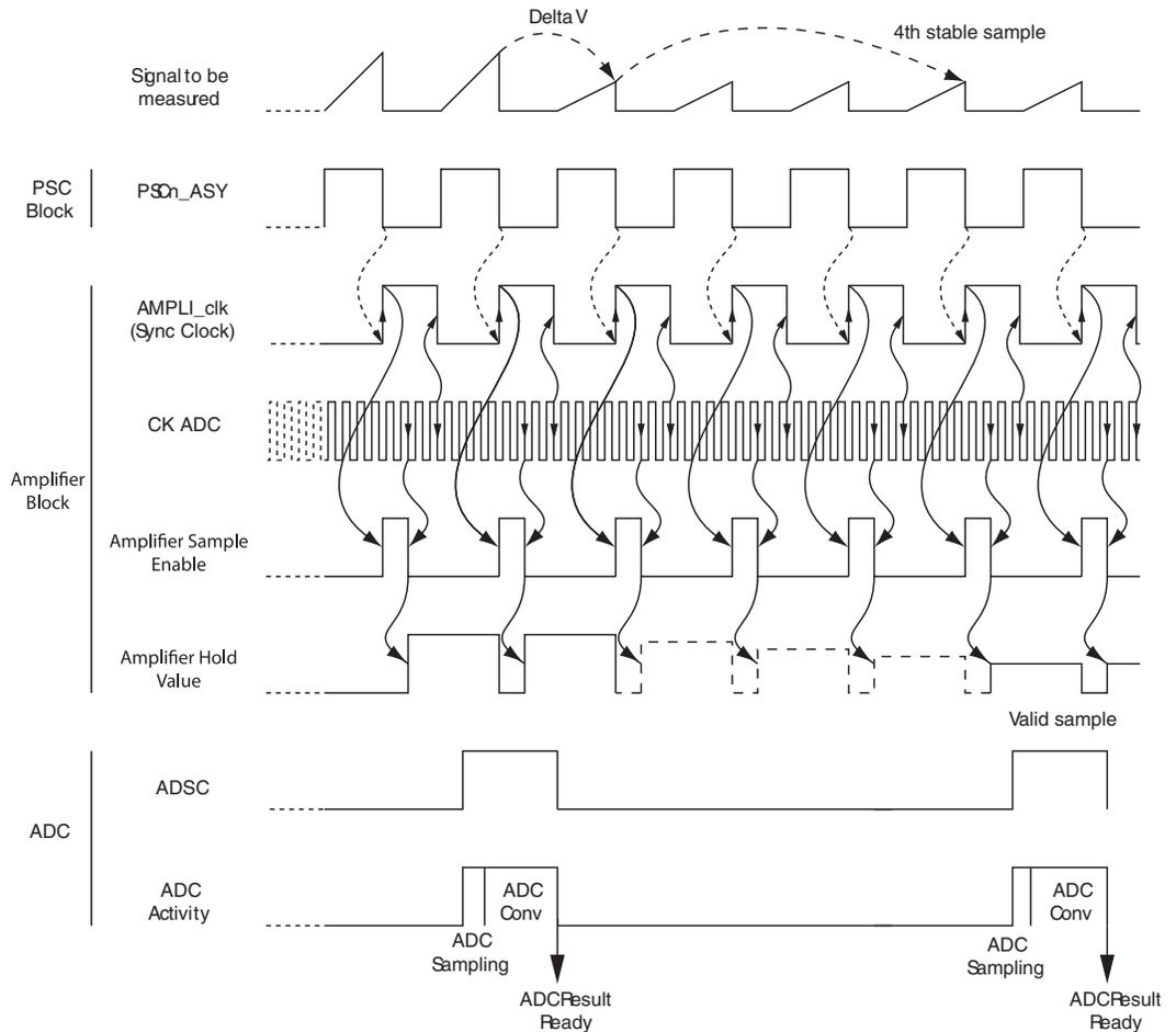
**Figure 21-17.** Amplifier synchronization timing diagram for AT90PWM2B/3B
