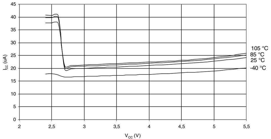
Figure 27-40. ADC Current vs.  $V_{CC}$  (ADC at 50 kHz)
