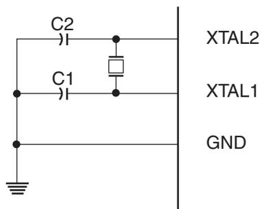
The Oscillator can operate in three different modes, each optimized for a specific frequency range. The operating mode is selected by the fuses CKSEL3..1 as shown in [Table 7-4](#).
