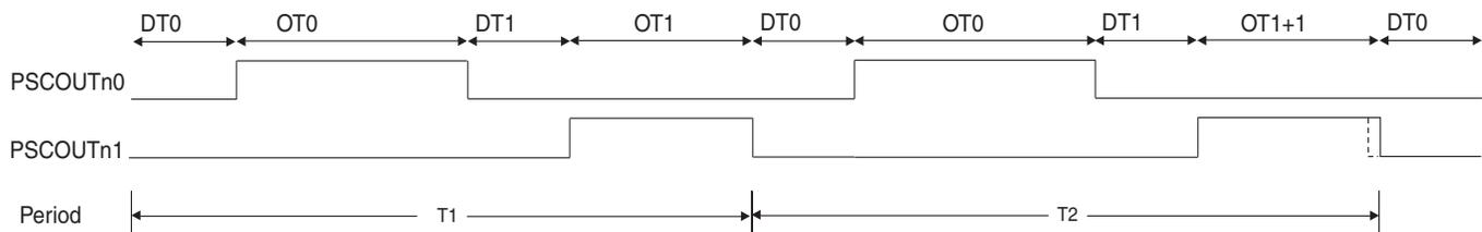
The supplementary step in counting to generate  $f_{b2}$  is added on the PSCn0 signal while needed in the frame according to the fractional divider. See [Table 16-5, "Distribution of fb2 in the modulated frame," on page 141](#).
