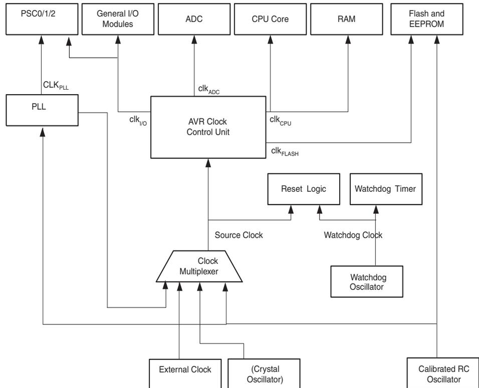
**Figure 7-2. Clock Distribution AT90PWM2B/3B**
