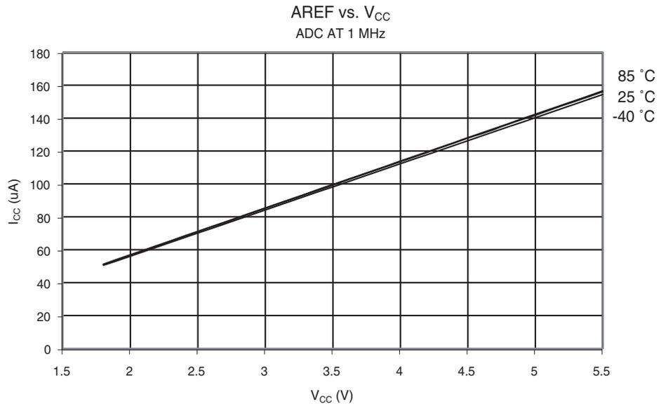
**Figure 27-42.** Analog Comparator Current vs.  $V_{CC}$
