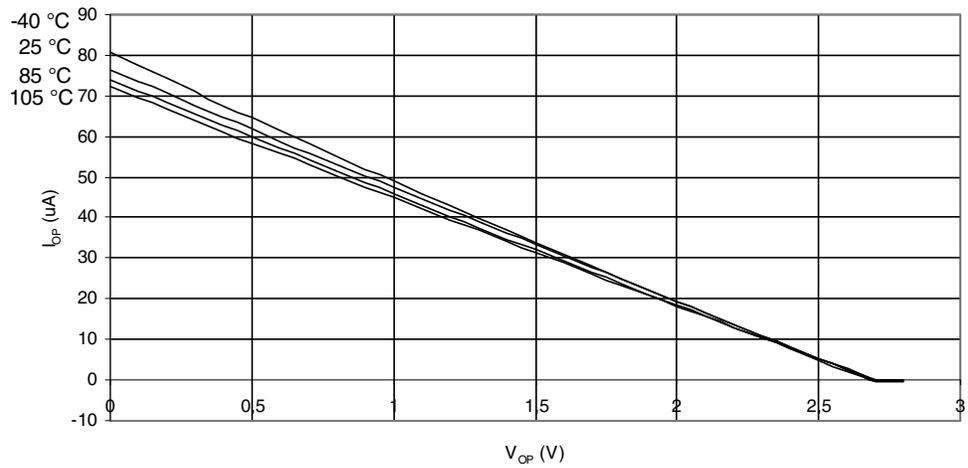
**Figure 27-13.** Reset Pull-Up Resistor Current vs. Reset Pin Voltage ( $V_{CC} = 5V$ )
