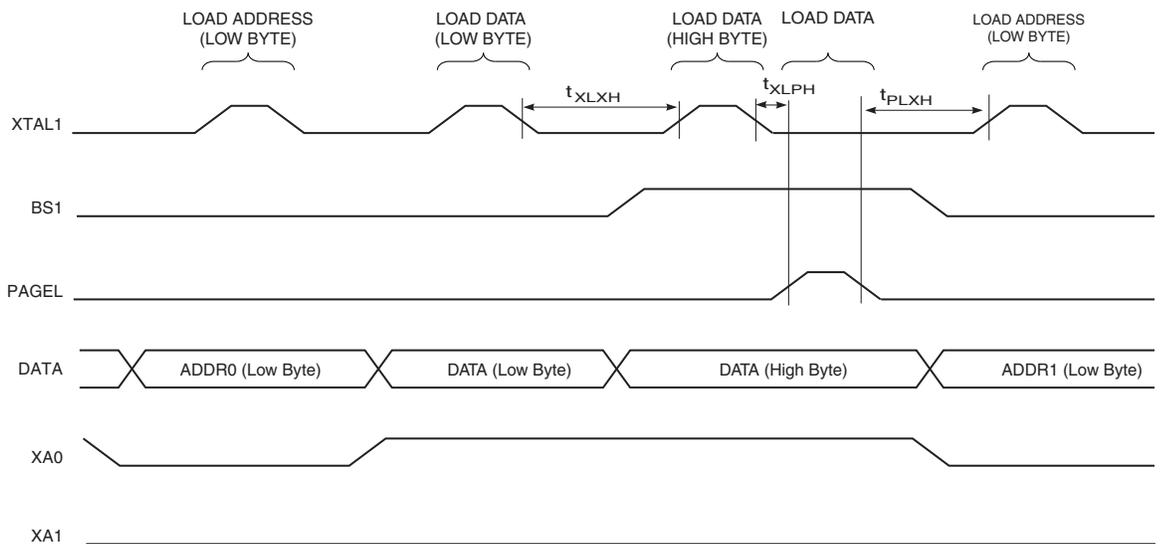
Note: 1. The timing requirements shown in Figure 26-5 (i.e.,  $t_{DVXH}$ ,  $t_{XHL}$ , and  $t_{XLDX}$ ) also apply to loading operation.
