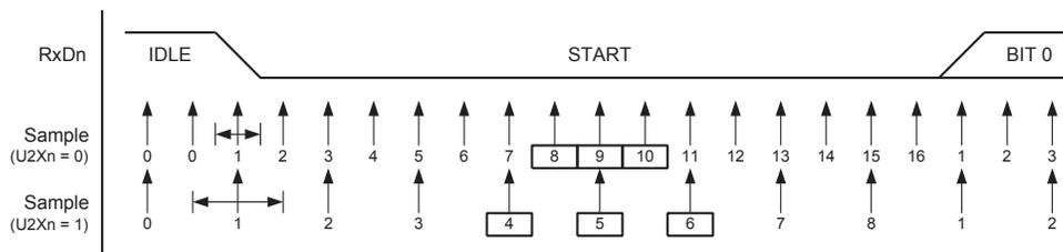
When the clock recovery logic detects a high (idle) to low (start) transition on the Rx/D line, the start bit detection sequence is initiated. Let sample 1 denote the first zero-sample as shown in the figure. The clock recovery logic then uses samples 8, 9, and 10 for Normal mode, and samples 4, 5, and 6 for Double Speed mode (indicated with sample numbers inside boxes on the
