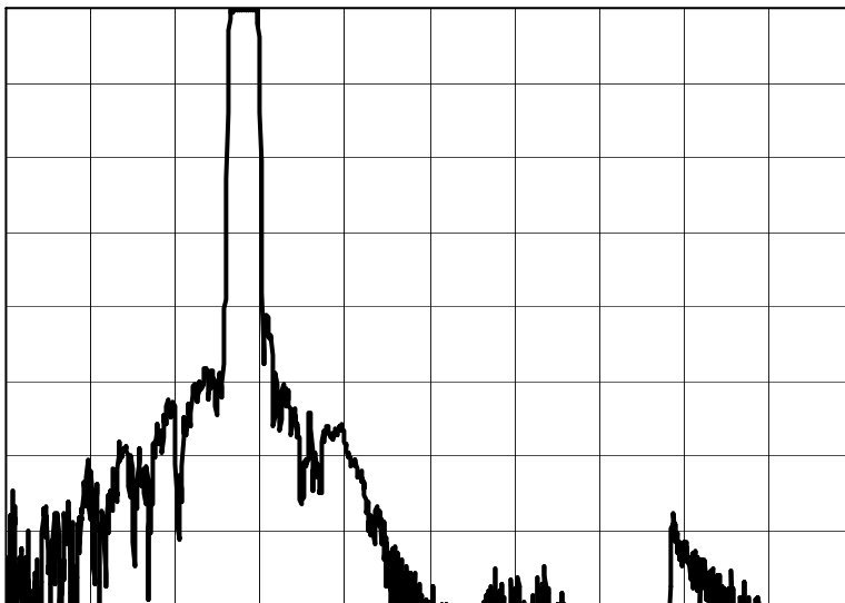
Wide Band Response Frequency Span : 0-500 MHz Vertical Scale : 10 dB/div
