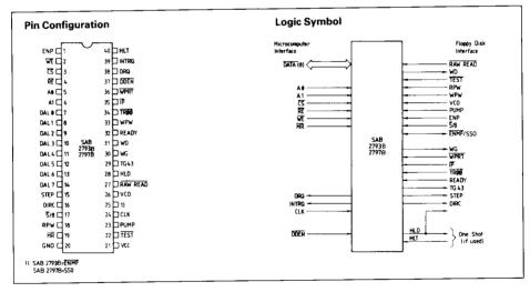
The SAB 2793B/2797B are floppy disk controllers in N-channel MOS LSI technology designed to interface with SAB 8080/8085/8051/8086/8088/80186/80188/80286 family processors. Its flexibility and ease of use makes it an ideal floppy disk interface between conventional floppy disks and all computer systems. Software-compatible with its predecessor, the SAB 179X, the device also contains a high-
