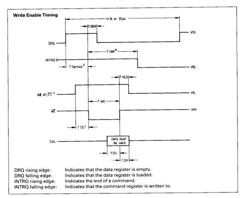
$<sup>^{11}</sup>$   $\overline{\text{CS}}$  may be permanently tied low if desired. When writing Data into Sector, Track or Data Register, the User cannot read this register until at least 4  $\mu s$  in MFM after the rising edge of  $\overline{\text{WE}}$ . When writing into the Command Register status is not valid until some 28  $\mu s$  in FM/14  $\mu s$  in MFM later. These times double when CLK = 1 MHz.
