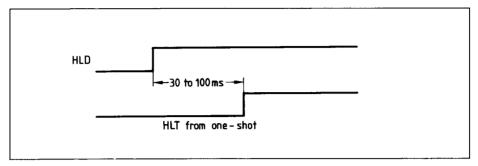
When both HLD and HLT are true, the SAB 2793B/2797B will read from or write to the media. The "AND" of HLD and HLT appears as status bit 5 in Type I status.
