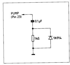
Since  $5^{1/4}$ " Drives operate at exactly one-half the data rate (250 Kbyte/s) the above capacitor should be doubled to 0.2 or 0.22  $\mu F$ .
