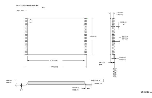
Figure 13. 48-Pin TSOP I (12 mm x 18.4 mm x 1.0 mm), 51-85183
