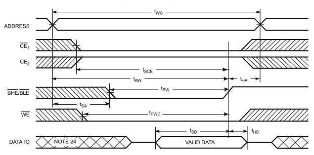
Figure 10. Write Cycle No. 4
