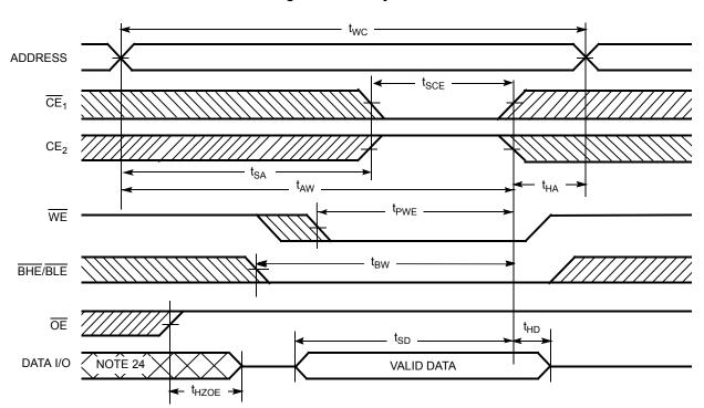
Figure 8. Write Cycle No. 2
