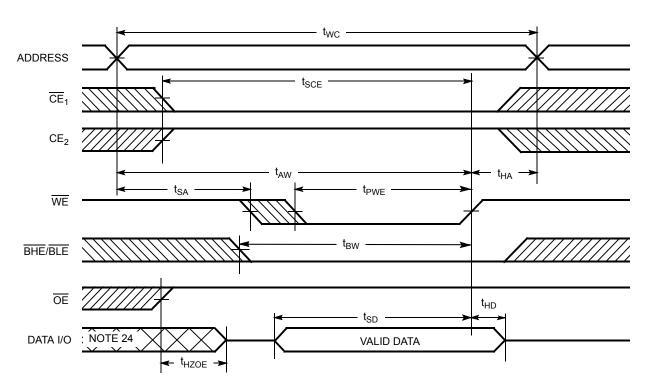
Figure 7. Write Cycle No. 1
