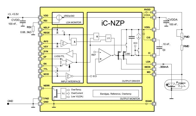
Figure 3: Circuit example for P-type laser diodes (case grounded)
