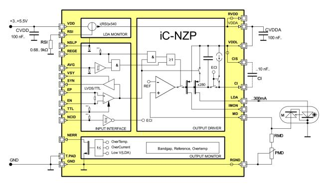
Figure 4: Circuit example for M-type laser diodes (case grounded)
