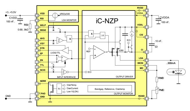
Figure 7: Example set-up for current control
