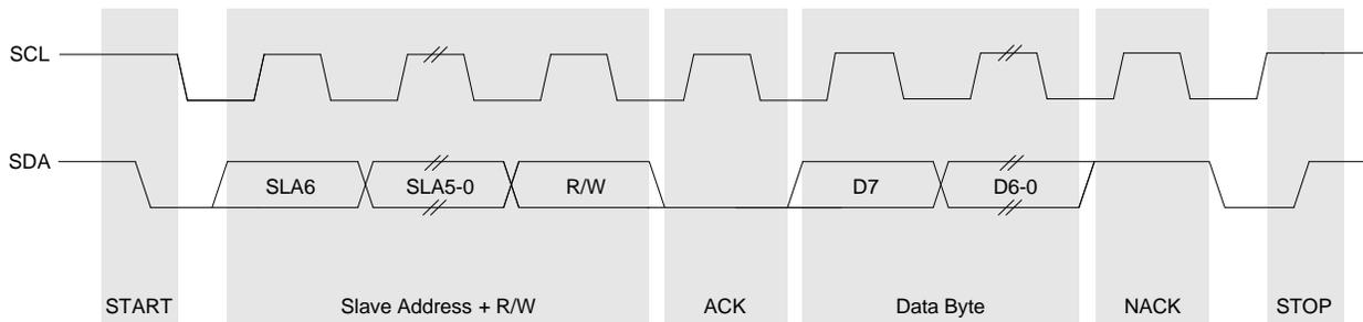
**Figure 5. I<sup>2</sup>C Bit Timing Diagram**
