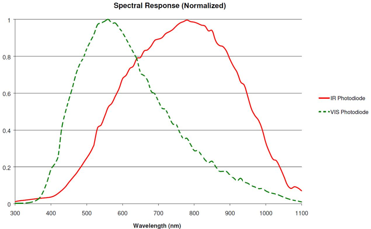
**Figure 4. Typical Ambient Light Sense Performance Curves (Preliminary)**
