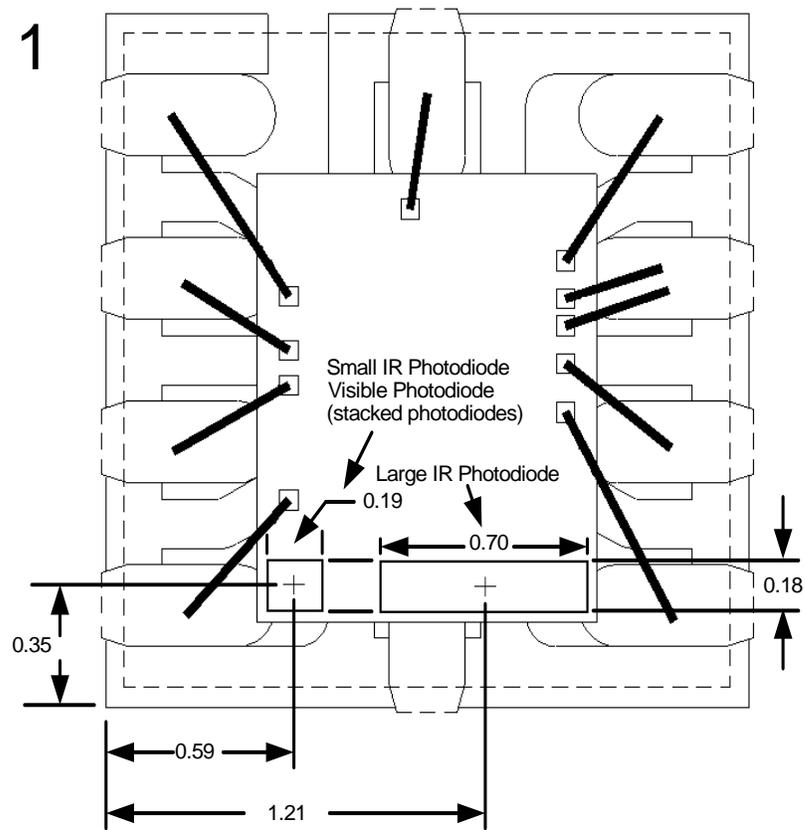
Figure 13. Photodiode Centers
