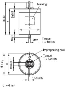
d<sub>1</sub> = 6 mm Creepage distance 12.7 mm min. Clearance 9.6 mm min.
