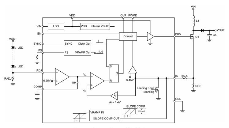
Figure 2. MIC3230 Functional Block Diagram
