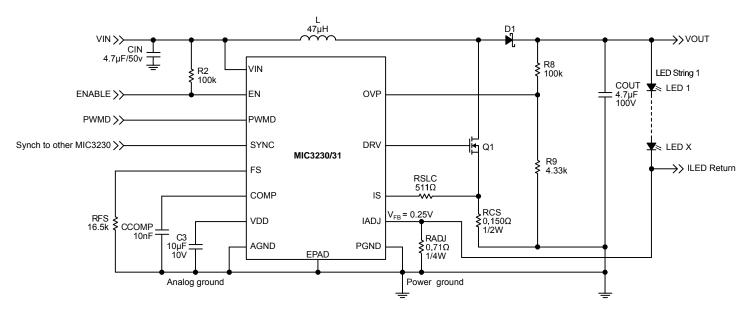
Figure 1. Typical Application of the MIC3230 LED Driver
