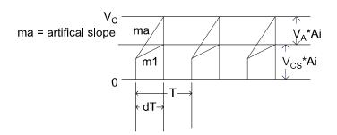
Figure 3. Slope Compensation Waveforms
