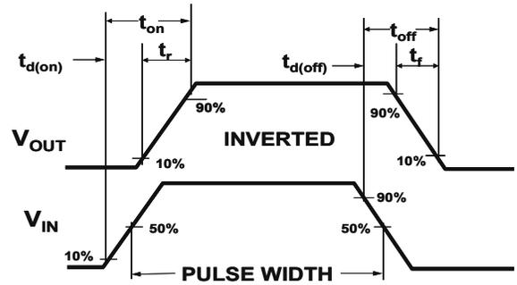
Figure 2: Switching Waveforms
