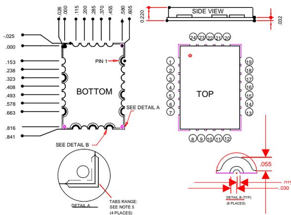
1. The inside radius of all 24 half holes at the perimeter of the board are plated to provide a surface for the attachment of the PLL Module to the PCB. 16 pads are for grounding, 8 pads are for signal interface.
