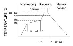
Figure 1. Re-flow Soldering
