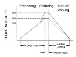
Figure 2. Iron Soldering
