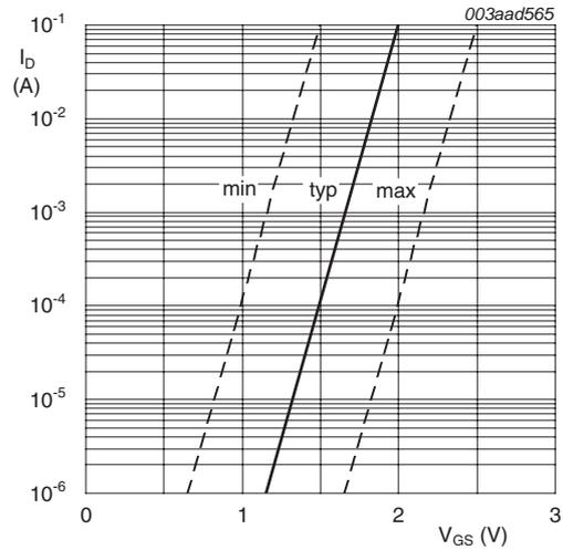
$$T_j = 25^\circ\text{C}; V_{DS} = V_{GS}$$
