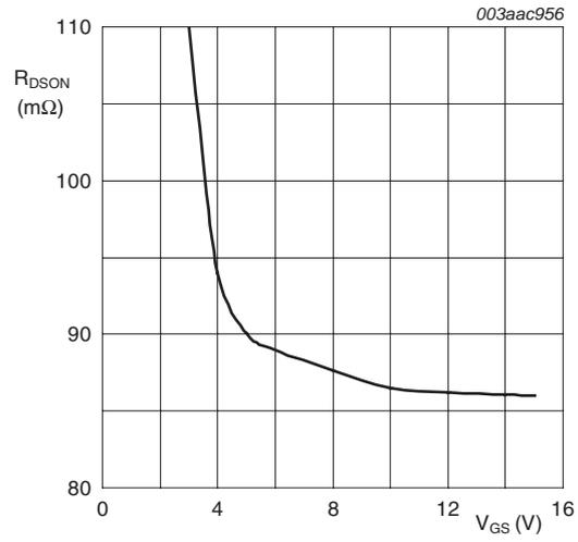
$$T_j = 25^\circ\text{C}; I_D = 5\text{A}$$
