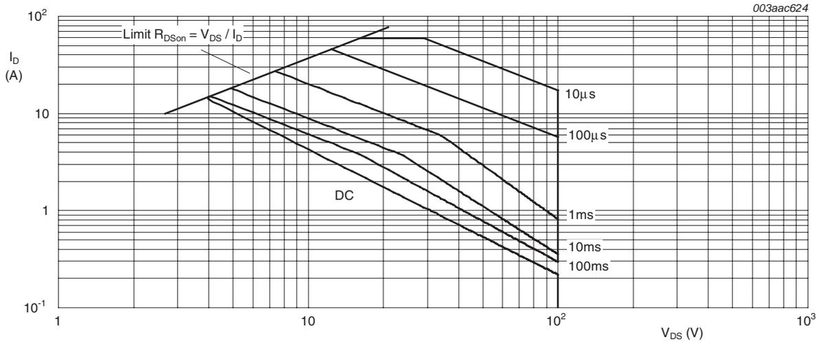
$T_{mb} = 25\text{ }^\circ\text{C}; I_{DM}$  is single pulse
