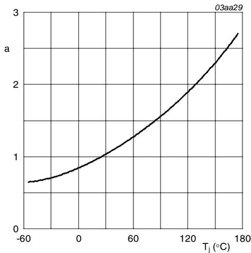
$$a = \frac{R_{DSon}}{R_{DSon(25^\circ\text{C})}}$$
