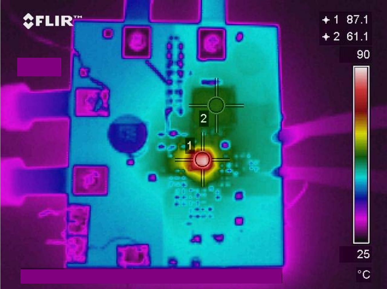
Fig. 17: Thermal Image at 12A load Test points 1 and 2 are IR3840W and inductor, respectively.
