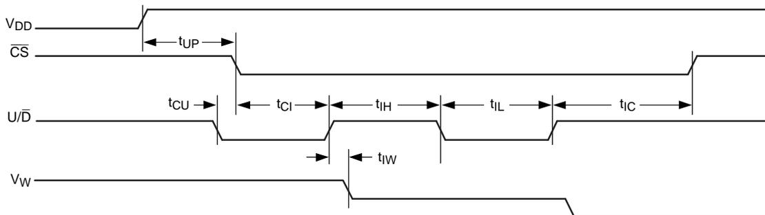
**Figure 2. Decrement Mode Serial Interface Timing Diagram**
