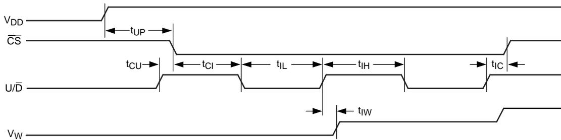
**Figure 1. Increment Mode Serial Interface Timing Diagram**
