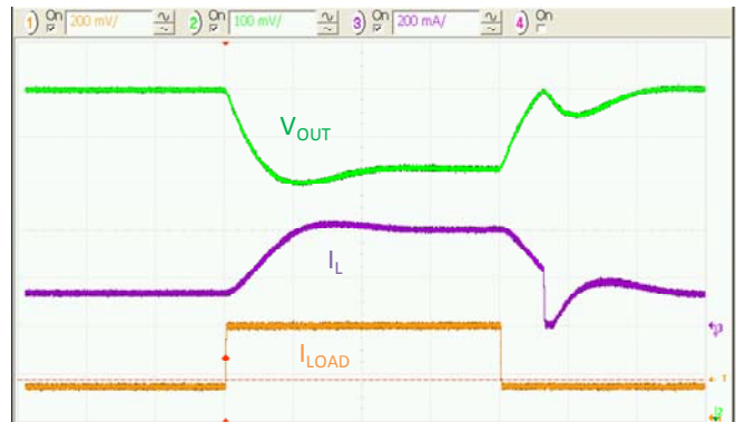
Figure 23. Load Transient 150mA to 400mA, V_{IN}=3V , t_{RISE}=t_{FALL}=100ns , 5\mu s/div .
