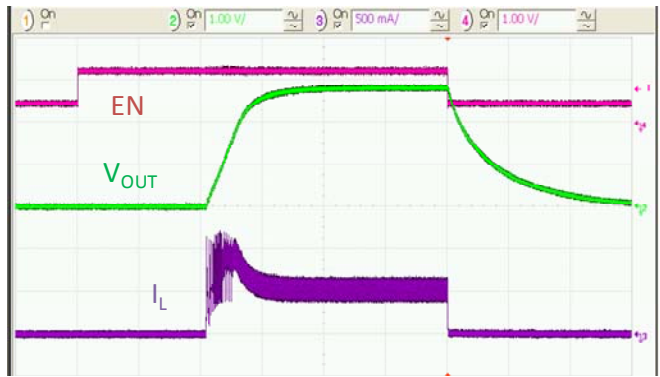
Figure 17. Startup and Shutdown through V_{EN} with 500mA Load, 50µs/div.
