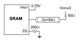
Note: Parameters are tested with RQ=250 $\Omega$
