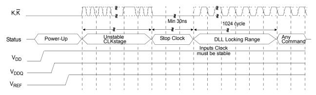
\* Notes: When the operating frequency is changed, DLL reset should be required again.
