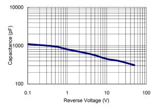
FIG 4 Typical Reverse Characteristics
