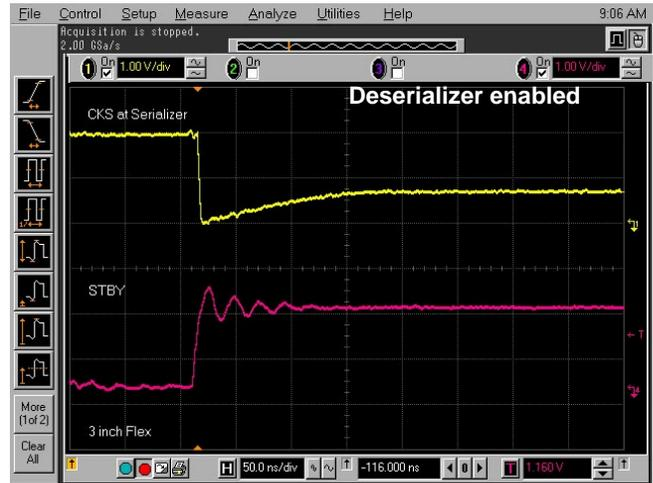
Figure 1 – CTL Enable Pulse
